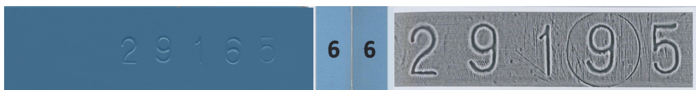
Punching of symbol, rotation, pressing in
